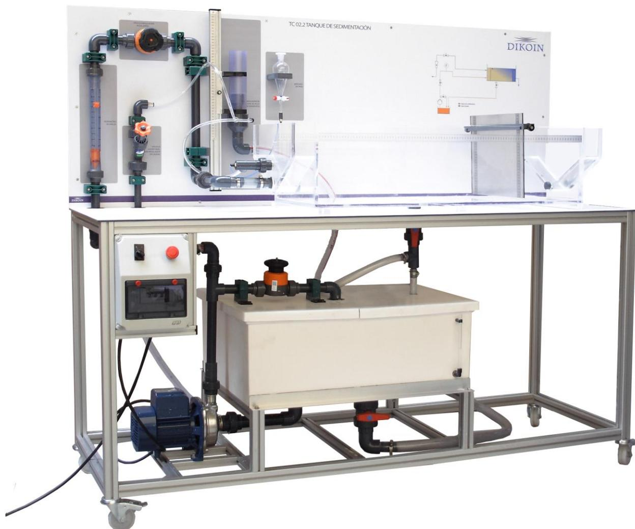
With this equipment is intended to study and visualize in a continuous regime, the natural phenomenon called sedimentation, whereby particles that are denser than the fluid that contains them and in which they are dispersed, fall by gravity depositing in the bottom of the container.
