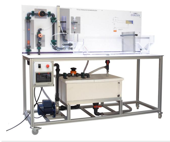
With this equipment is intended to study and visualize in a continuous regime, the natural phenomenon called sedimentation, whereby particles that are denser than the fluid that contains them and in which they are dispersed, fall by gravity depositing in the bottom of the container.
